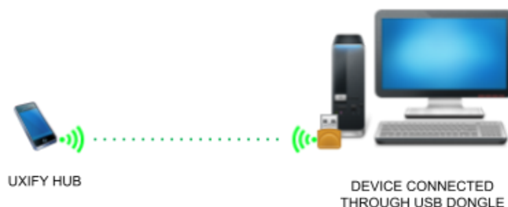
Figure 7: USB dongle enables connection between UXify Hub and a desktop
